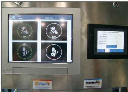
**Vision displays data in a user-friendly interface** and automates product rejection, or stops the line.
